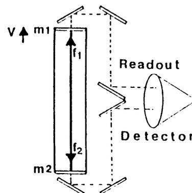
Figure 3. Laser speedometer.
