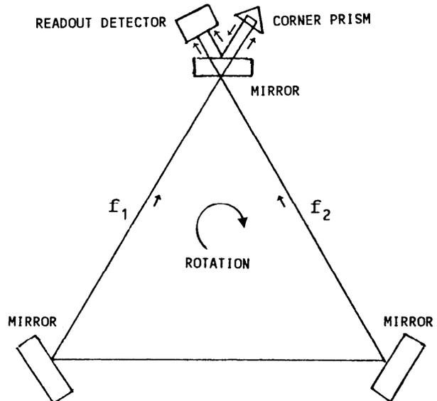
Figure 2. Laser gyro beam paths.
